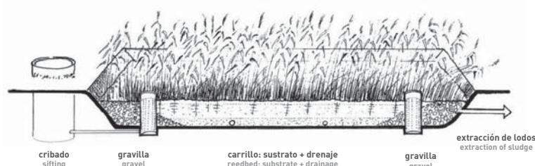
2. filtro plantado de flujo vertical vertical-flow planted filter
